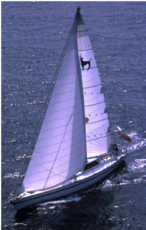
A 120-percent-overlap working jib on a Deerfoot 74. The sheet lead has been moved forward from the beating position for reaching, resulting in an even luff shape all the way up the sail.
