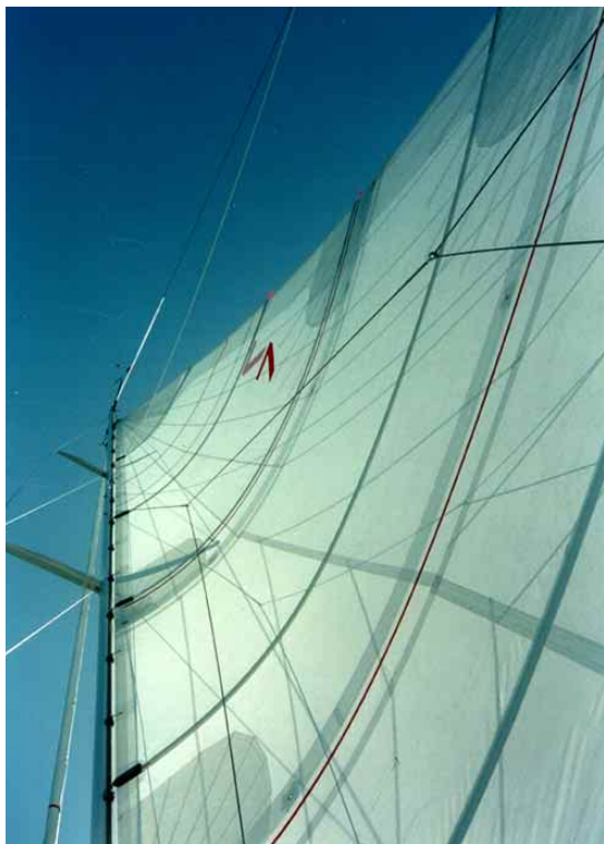
A nice-looking full-batten main with a conventional roach. The gently rounded leading edge and straight leech make it both easy to trim and fast. (North Sails RI photo)
