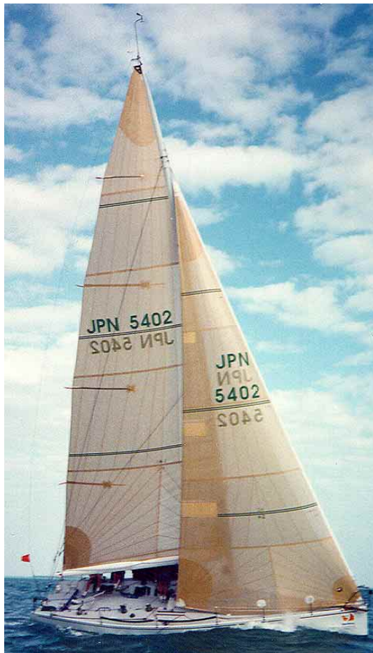
Radial construction has been made efficient by modern sailcloth and computer-aided design for panel layout and cutting. (North Sails RI photo)
