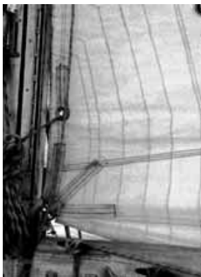
The tack and cunningham on Sundeers mainsail are heavily reinforced. Note the many layers of Dacron plus webbing.
