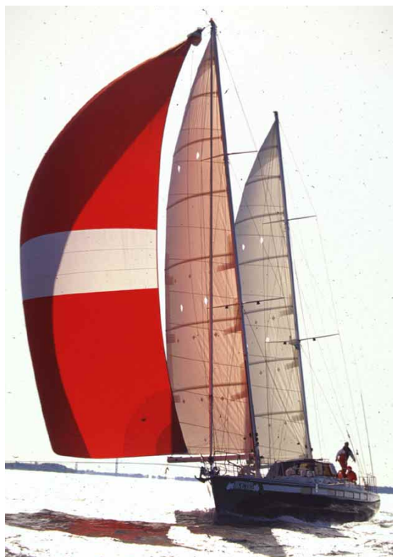
A nice-looking asymmetrical on the Sundeer 64 Artemis . John Conser cut this sail more for broad-reaching and running than close-reaching, although it could be flown as close as 55 degrees apparent. For really deep running, however, the sail would fly much better if tacked off a spinnaker pole.
