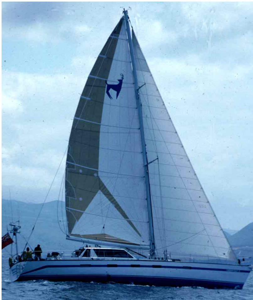
The overlap on this main past the backstay is 28 inches (711 mm). That looks and sounds like a lot, but today we are much more aggressive with the roach.
