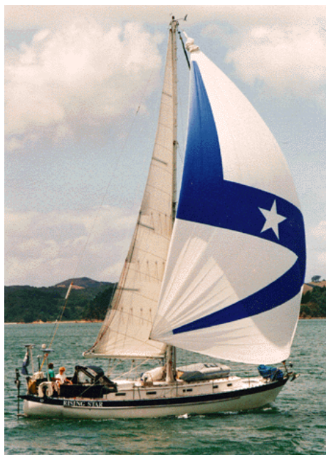
A modern cruising chute on a Valiant 42. Compare how much fuller this sail is than the one on the preceding page. It can be used down to angles as deep as 140 to 150 degrees. Beyond this it will become very difficult to fly unless poled out. (Port Townsend Sails photo)
