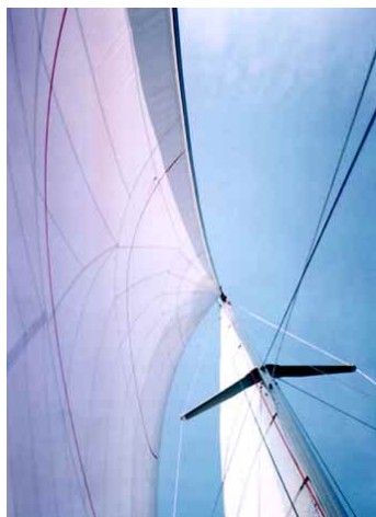
The padded luff on this roller-furling jib (left) creates bulk when the sail is rolled, which in turn tends to flatten the sail. (North Sails RI photo)
