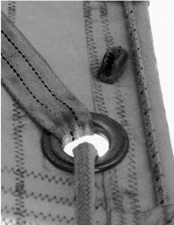
A D-ring webbed onto a reef clew (above right) with a combination of Kevlar (it's a Kevlar sail) and Spectra webbing.
