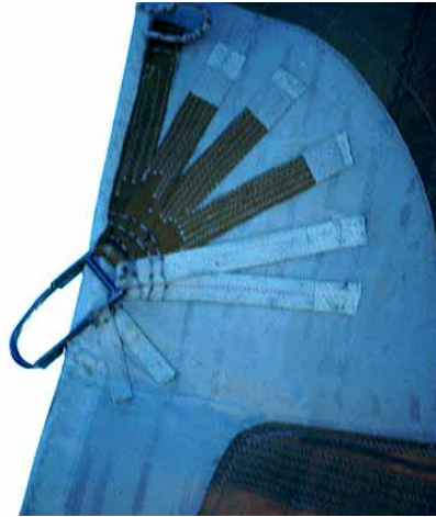
A D-ring webbed onto a reef clew (above right) with a combination of Kevlar (it's a Kevlar sail) and Spectra webbing.
