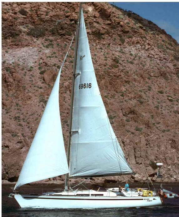
Bruce Farr has been putting fractional rigs on cruising boats since the late 1970s. Beach Party , a Kiwi-built 46-foot (14.2m) yacht, has typical proportions for one of his boats. Note how far forward the main mast is, and how large the main is relative to the jib.
