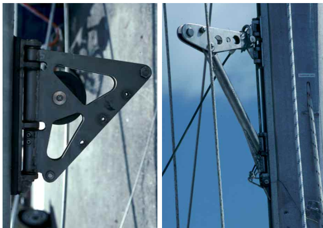
Two very sophisticated approaches to headboard attachment. The system on the left incorporates a sheave for a 2-to-1 halyard. In both cases the headboard is pinned at the top and bottom of the carrier.
