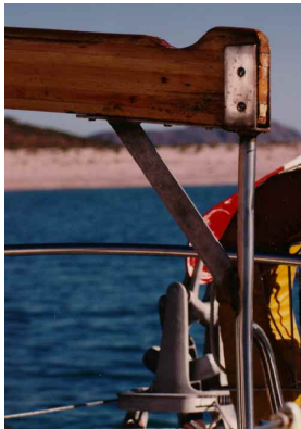
Tim Traill demonstrates how his boom gallows provide security and support for the helmsman. They are relatively easy to execute — just be sure
