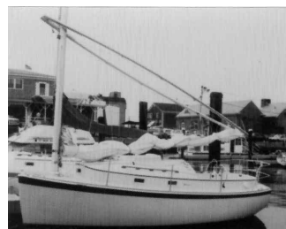
Eric Sponberg sent us these photos of the Nonsuch 22 for which he designed the freestanding rig. The wishbone boom is particularly interesting. Because it is angled down, it serves as a vang as well as the boom, automatically controlling leech twist.
