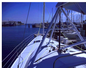
The B&R tripod (above) spreads the mast load into the hull and reduces the required length of the mast. (Lars Bergstrom photos)
