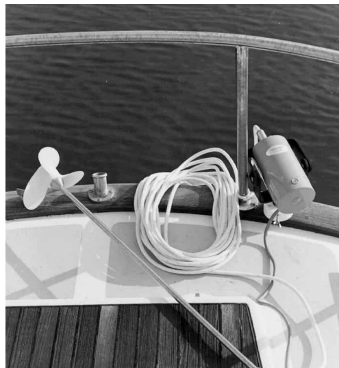
The Ham Ferris rig shown here has provided power on many passages. Just remember to mount it on the port side, so prop torque walks the prop and line out away from the boat. If it is mounted to starboard it will eat any fishing lines or taffrail logs streamed from the port side. (Sea Air Land Technologies photo)
