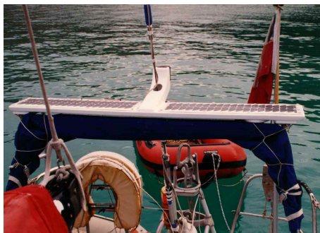
Above and left are installations that have trouble with shading. The radar and miscellaneous antennae will cut output significantly.
