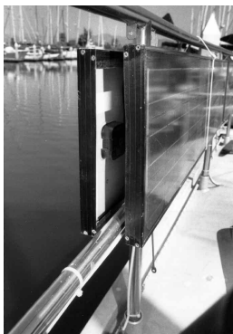
Three views of the eight panels on Sundeer . (above and left) Over several years of cruising we found that these provided about 15 amp hours per panel per day (at 12 volts). Four of the panels would stay even with the fridge/freezer if we left the boat. But opening and closing the fridge/freezer doors this would jump us up to six panels.
