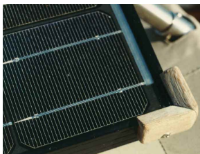
Sharp corners on panels (above and below) can be a danger to crew and sails. These need to be filed down, or better yet, covered with a timber cap.
