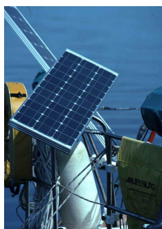
Three adjustable installations (above). If space is limited and you can't find room for a third panel, it makes a difference to be able to tilt and manually track.
