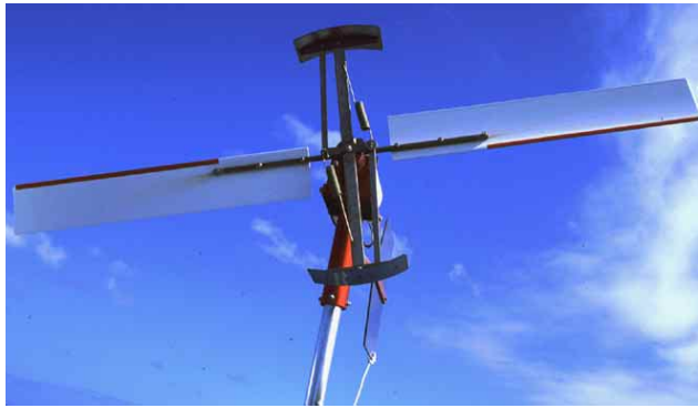
These two photos show the over-speed brake on a Four Winds windmill. This unit, like most U.S.-made windmills, is based on a DC motor.
