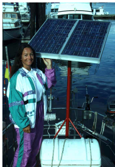
Three adjustable installations (above). If space is limited and you can't find room for a third panel, it makes a difference to be able to tilt and manually track.
