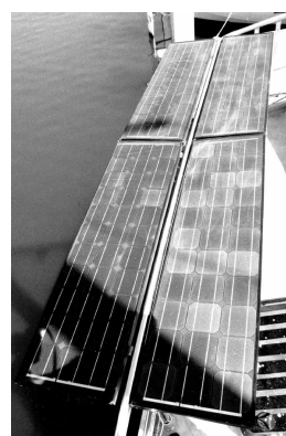
Three views of the eight panels on Sundeer . (above and left) Over several years of cruising we found that these provided about 15 amp hours per panel per day (at 12 volts). Four of the panels would stay even with the fridge/freezer if we left the boat. But opening and closing the fridge/freezer doors this would jump us up to six panels.
