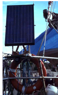
Three adjustable installations (above). If space is limited and you can't find room for a third panel, it makes a difference to be able to tilt and manually track.
