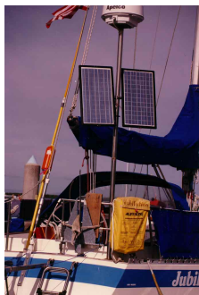
Here are two simple installations (above) that can be made to manually track the sun as well as have the correct angle of declination. Both are simply supported on a single aluminum pole. Note the simple attachment hardware in the right photo.
