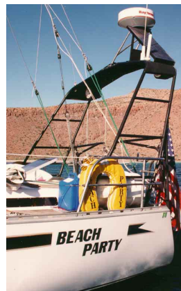
Above and left are installations that have trouble with shading. The radar and miscellaneous antennae will cut output significantly.
