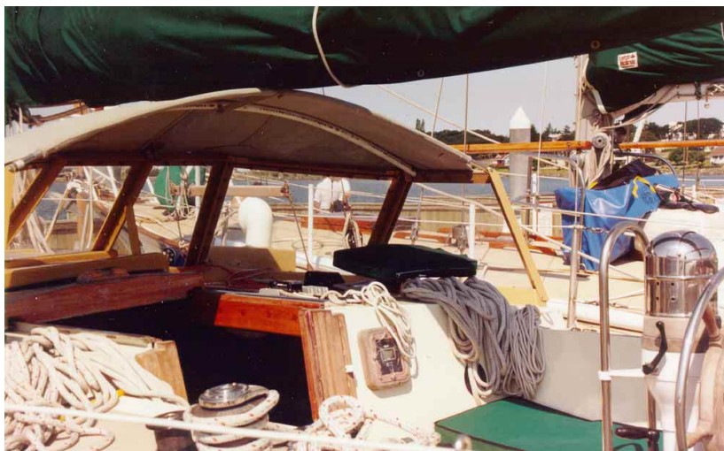
A short hard top like this is quite popular on European boats. It does provide good protection for the companionway hatch, but the crew is pretty much left out in the rain and spray unless the hard top is extended in some form of top and side curtains.
