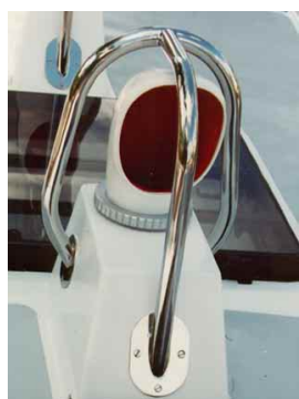
A stainless dorade cowl, now available from Bomar (left), compared to the Vetus Yogi-style cowl (right). There is probably twice the cowl
